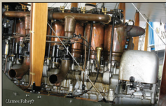
The same engine after a few hours flying time. Note the extensive oil staining and patina of the copper water jackets and intake pipes (E24) and the protective magneto cover (E17).
