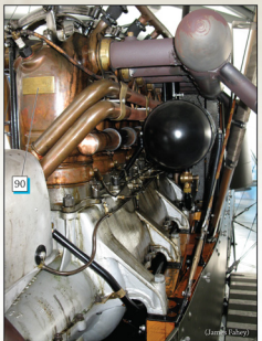
^ > Rear right view showing the position of the oil tank (E8) & (E20) under the late style silencer (E29) & (E31).
