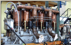
160hp Beardmore engine #2192 is readied for TVAL FE.2b 6341. Note the oil pump (E21) at left.
