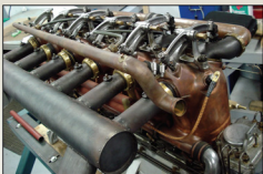
Top view showing the rocker arms, water outlet pipe and cylinder water jackets before being mounted into TVAL FE.2b 6341.
