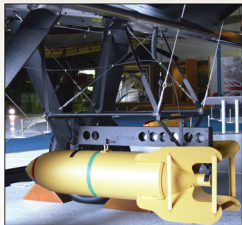
230lb HE RFC bomb Mk.1 fitted to its 230lb Bomb Carrier single Mk.1 under Hendon's FE.2b A6526.
