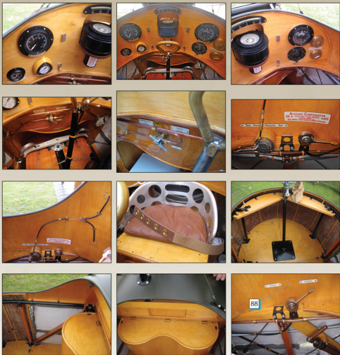
Interior detail photos from TVAL FE.2b 6341. While some details of the 'Pilot's Locker' cockpit arrangement are not suitable for this model, many interesting details can be seen in these photos.
